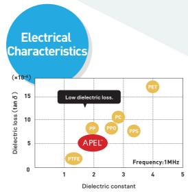
APEL<sup>™</sup> has characteristics of low dielectric loss and low dielectric constant
