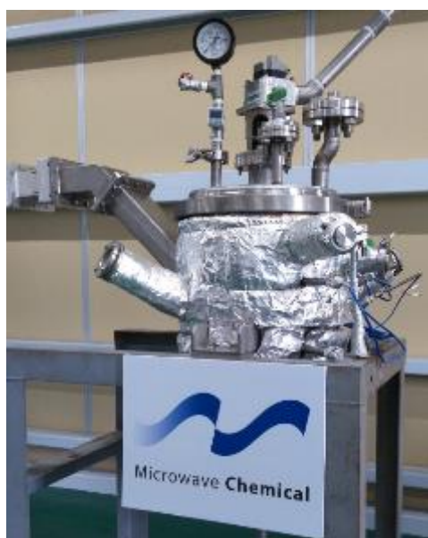
Small microwave demonstration device for decomposition of plastics
